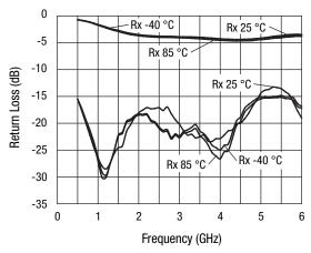
**Return Loss Rx Isolation State vs. Frequency**
