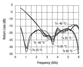
**Return Loss Tx Isolation State vs. Frequency**
