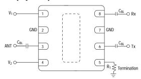
$C_{BL} = 39 \text{ pF for operation} > 500 \text{ MHz}.$
