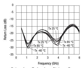
**Return Loss Tx Ins. Loss State vs. Frequency**
