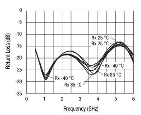
Return Loss Rx Ins. Loss State vs. Frequency
